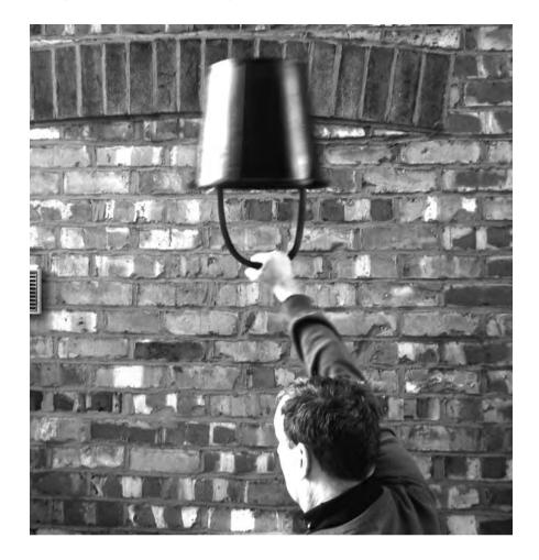
The bucket is half filled with water and swung. The water stays in the bucket, even at the top of the circular path, as long as the speed of the bucket exceeds a certain value.
